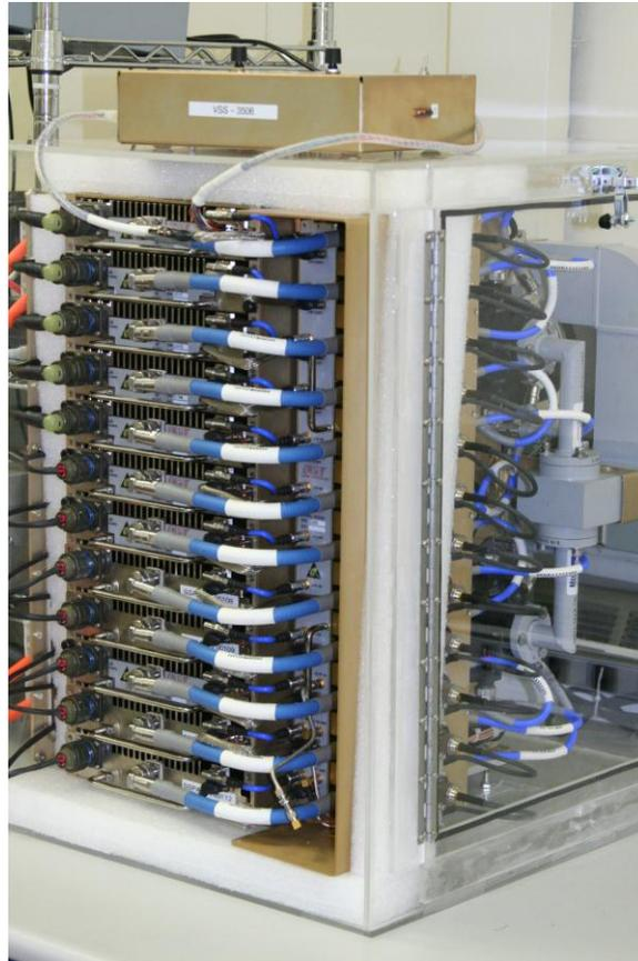
**Figure 10 VSS3605 SSPA under test at CPI**
