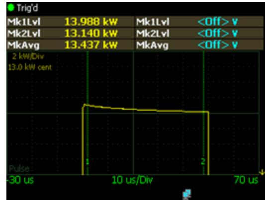
**Figure 15 Power at 20 usec pulse width at 1 kHz pulse repetition frequency**
